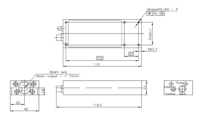
Sizes — in mm Tolerance— ± 0,2mm
